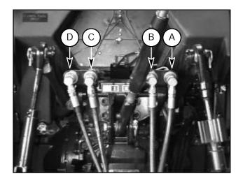
Figure 7. Hose Connection to Tractor
